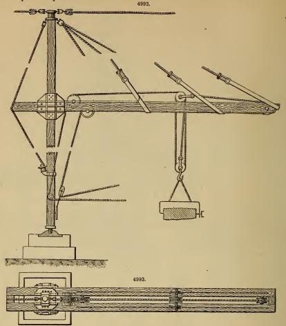
When the load is suspended at the end of the crane, the vertical brace is subjected to a tensile strain, which is provided for by its attachment to the iron shoes at the ends. To resist the torsional strain in the saddle, caused by the diagonal draught of the main chains, an arm is projected some distance from the saddle, and carries a roller, Fig. 4996, that presses upon the inside of the framing, and relieves the main track. The sheaves and general tackle are of the ordinary construction.
